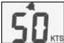
Alarm is on Wind alarm speed 50 kts (flashes)
