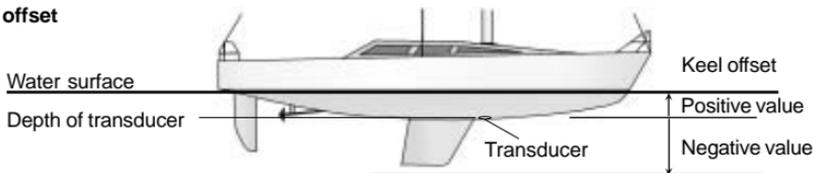
**Note:** The boat illustrated uses a through hull transducer
